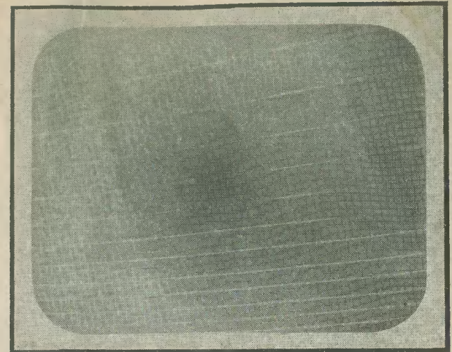
Fig. 1: The effect of ion burn on the screen is clearly shown here.
